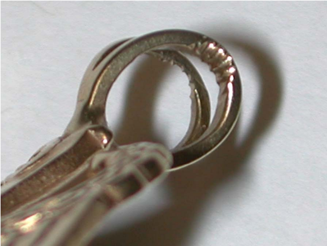
Gold bale on pendant after six years of wear
