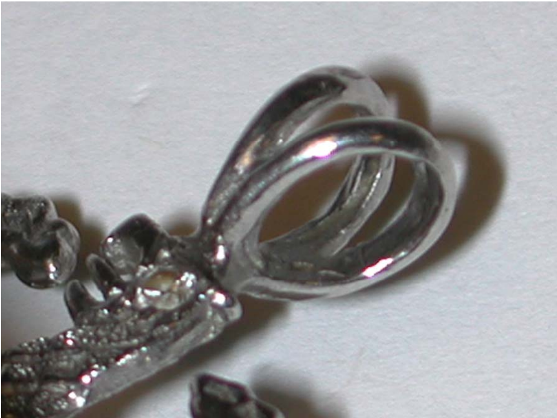
Platinum bale on pendant after six years of wear
