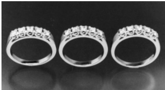
Fig. 1: (Left to right) Finished "fishtail" ring mountings in Pt-Co, Pt-Ru, and Pt-Ir alloys.
